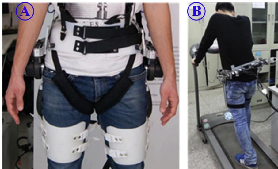
**Fig. 4.** Robotic hip exoskeletons for gait rehabilitation. (A) The robotic hip exoskeleton APO actuated by SEAs that comprise electric motors, custom torsional springs, harmonic drive, and a four-bar mechanism (Image credit: Elsevier); (B) the robotic hip exoskeleton actuated by electric motors through flexible Bowden cable transmission (Image credit: Professor Wang of the Southeast University, Nanjing, China).
