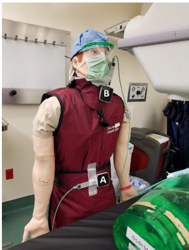
Figure 3. Clinical image depicting the mock surgeon positioned adjacent to the anthropomorphic pelvic model with scatter radiation measurement devices arranged for recording radiation exposure at the (A) body and (B) thyroid.
