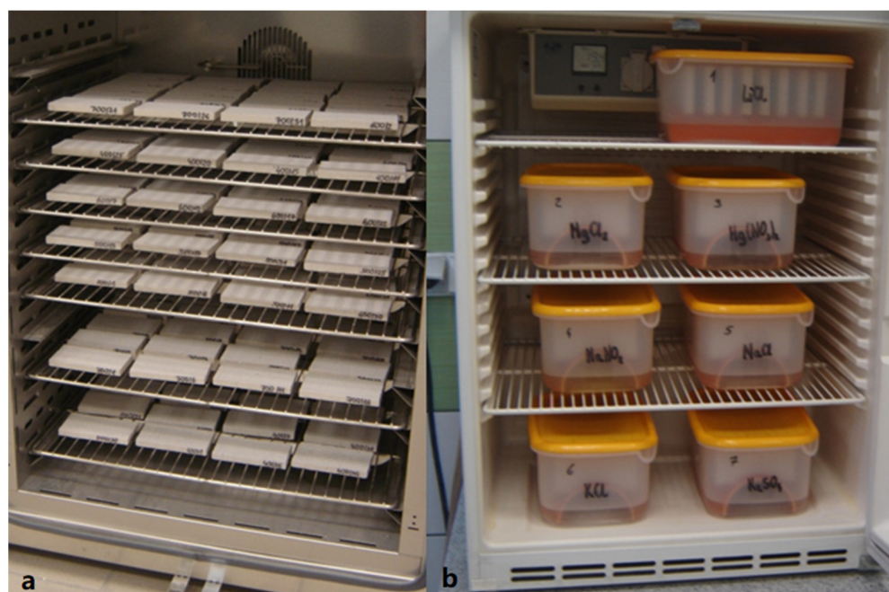
Figure 6. Samples dried to a constant mass, located in the dryer (a) and samples in closed containers placed inside the thermostatic chamber (b). Both photographs are from the authors' collection.
