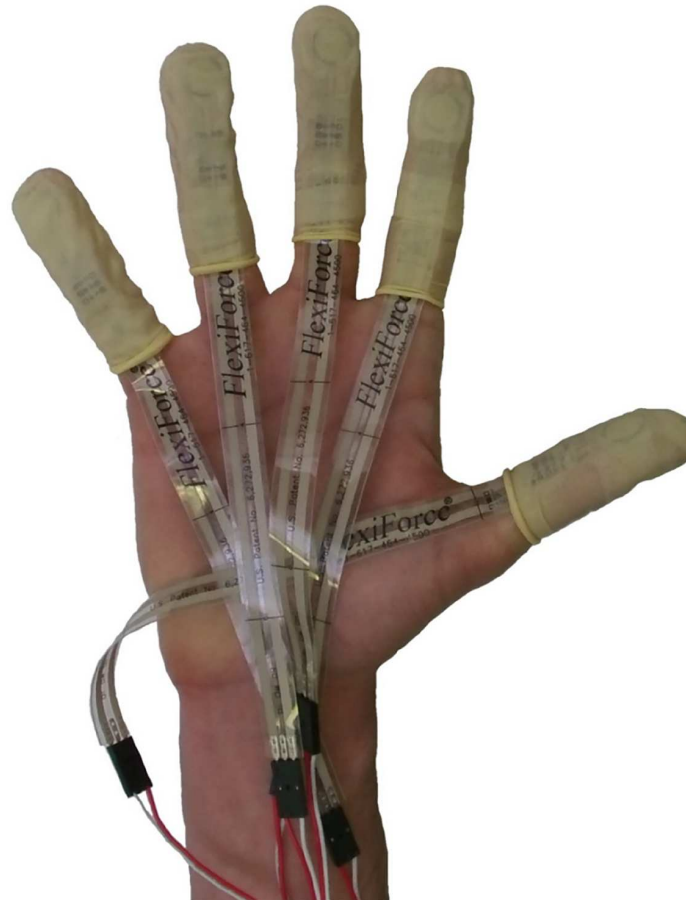
Fig 3. The Tekscan FlexiForce ® force sensors and where they were attached on the hand. The positioning of the circular (9.5mm diameter) pressure sensitive area upon the volar pad of each digit can be seen through the finger cots.
