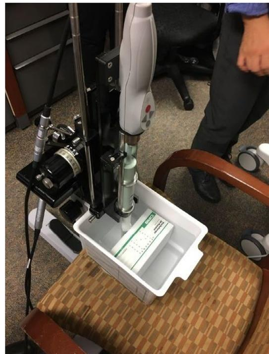
**FIGURE 8** Spatial resolution and accuracy measurements were performed using the experimental setup where a CIRS 045B phantom is submerged in room-temperature distilled water and set firmly against the ultrasound probed straddled in between the legs of an office chair where the water tank rests
