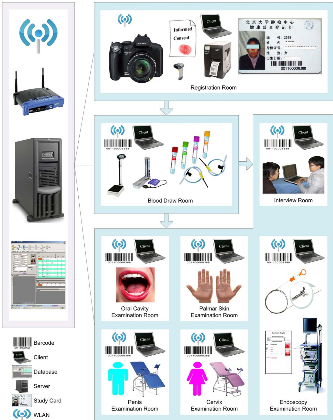
Figure 2. Computer-aided survey system (CASS) with client/server mode using a WLAN. The hosting system for the database resides on the server. The staff in each examination room can synchronously enter data in the database by logging into client application software installed on client computers using a wireless local area network (WLAN). After registration, blood is drawn. Eligible participants with no communicable blood diseases then continue on and participate in an interview and examination of the oral cavity, palmar skin, cervix/penis and esophagus. doi:10.1371/journal.pone.0031602.g002
