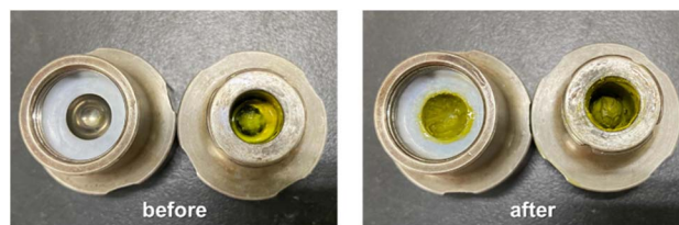
Fig. 3 Reaction mixture before and after ball milling (entry 1, Table 2).
