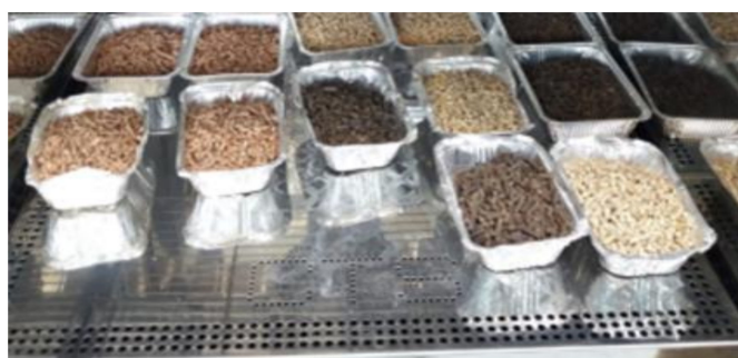
Figure 1. Pellets on aluminum trays in the climate chamber. This figure is an example showing the pellets on aluminum trays. The same trays were used for the other storage conditions.
