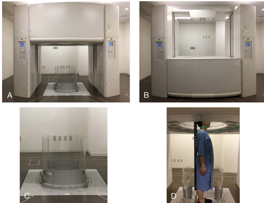
FIGURE 1. Upright CT machine and tools for safety. Our upright CT system enables up-and-down movements with a transverse 320 row-detector gantry. A, Gantry in the up position. B, Gantry in the down position. C, Knee-high acrylic wall encircling the body. D, Pole to lightly support the back of the patient.
