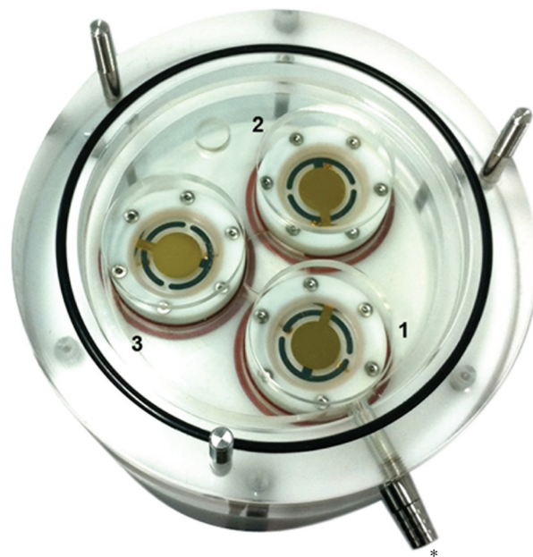
FIGURE 1: British American Tobacco's standard exposure chamber used for in vitro exposures to whole smoke at the air-liquid interface was modified to accommodate the 3 QCM units. The picture shows a top view of the 3-in-1 QCM exposure chamber base (crystal \phi = 2.54 cm; cell support insert \phi = 2.4 cm). QCM position 1 is proximal to the passive exhaust port *. QCM positions 2 and 3 are distal to the exhaust port and behind position 1 on the right and left, respectively.
