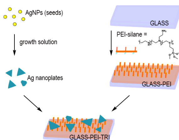
Scheme 1. A schematic representation of the synthetic route to polyethylenimine (PEI)-functionalized glass with citrate-capped Ag nanoplates (GLASS-PEI-TRI) samples.
