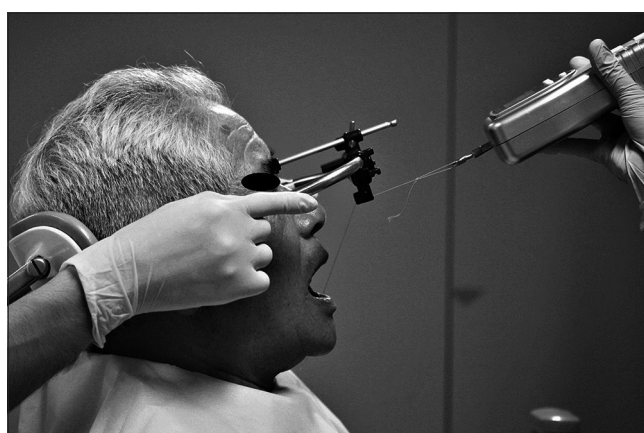
Figure 2: Standardized setting for measuring retention of the removable mandibular prosthesis. The denture is pulled out with a nylon thread by a force gauge through a facebow, pulling in parallel with the facebow arms. The facebow was positioned on the patient's face, and the facebow arms were firmly held in position by an assistant
