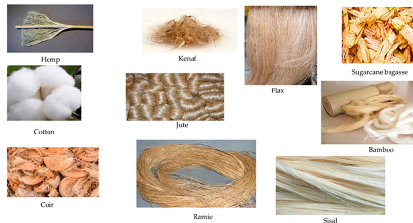
Figure 3. Different types of natural fibers. Reproduced with permission from Ref. [32].
