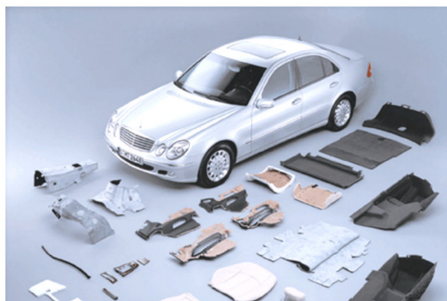
Figure 10. Car components are made up of natural fiber-reinforced composites. Adapted from reference [112] with permission.
