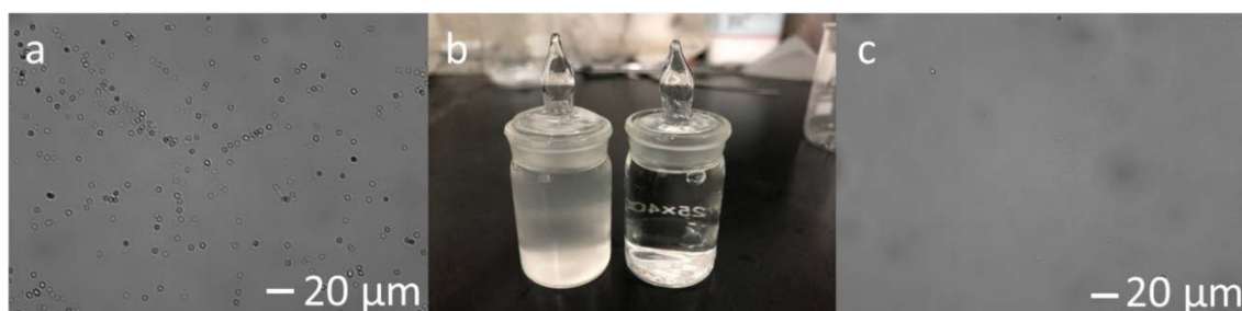
Figure 10. The beaker with oil-in-water emulsion (left-hand side in (b)), the beaker with water filtered through the membrane S1350-1650 at 0.1 MPa, 2.5 L/min (right-hand side in (b)), and the corresponding images from an optical microscope of the emulsion (a) and the filtered water (c).
