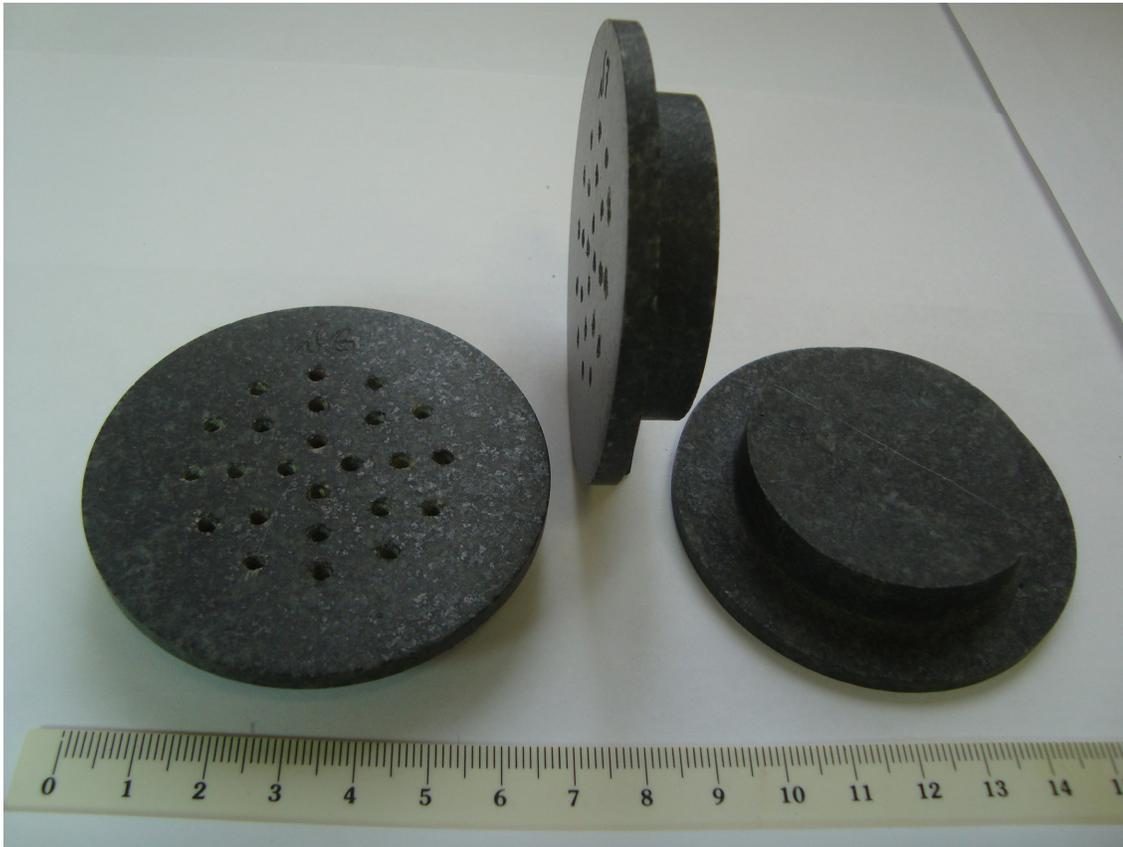
**Fig 1. The basalt discs before loading with microbial cultures.**
