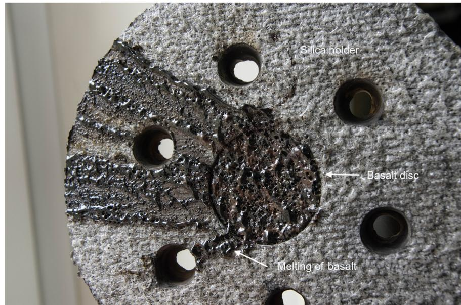
**Fig 4. Exterior of the test basalt disc (Disc #1) exposed to atmospheric entry.** Note the melting of the basalt.
