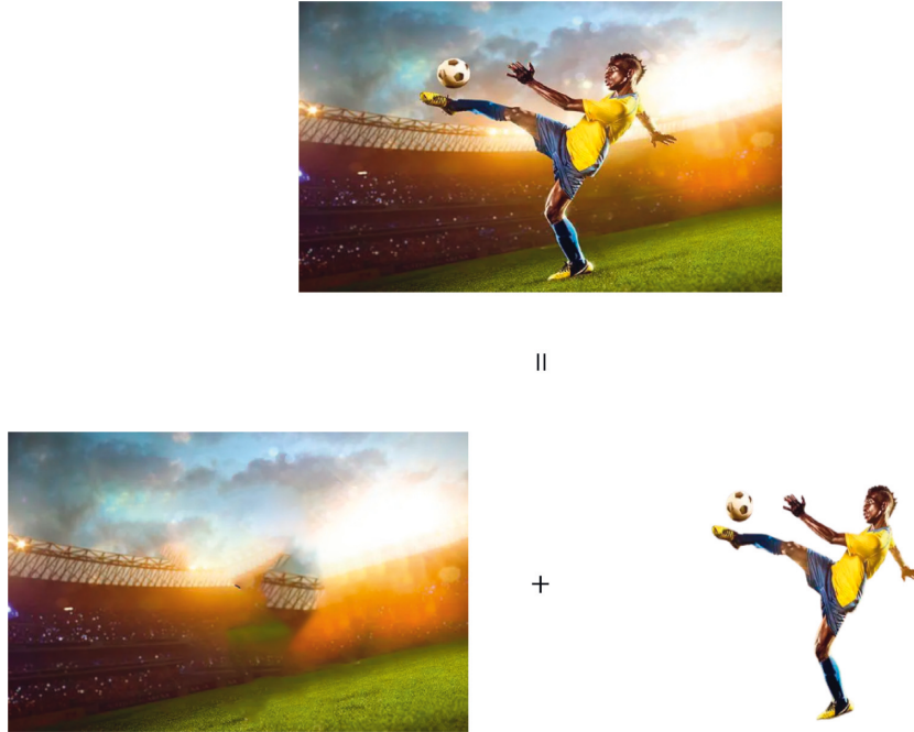
FIGURE 6: Schematic diagram of background difference method.
