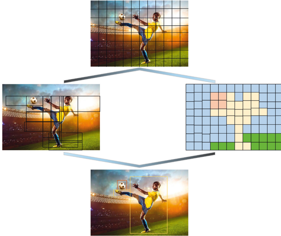
FIGURE 1: The principle of YOLO target detection.
