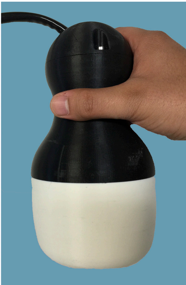
Figure 1. Photograph of the hybrid gamma camera.
