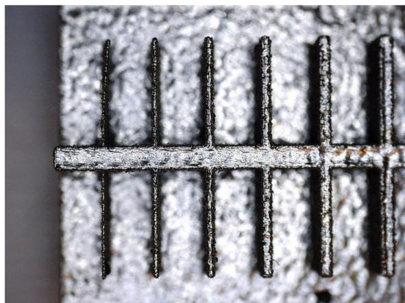
**Figure 27.** Presentation of the deformation of a fragment of a detail of a rectangular model made in the DMLS technology.
