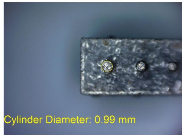
**Figure 11.** Measurement result for cylindrical holes and solids made in the DMLS technology: cylinder with a nominal diameter  $D_m = \text{Ø}1$  mm ( $D_{m1} = 0.99$  mm).
