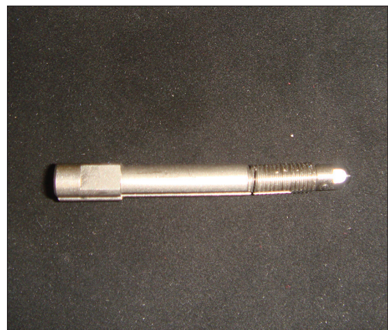
Figure 18: Broken distractor rod with a crack in its shaft noted at the time of distractor removal. This breakage seemed to have no influence on the distraction outcome
