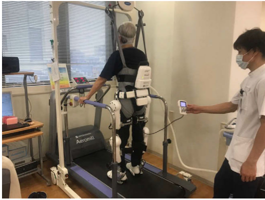
Figure 1. Gait training using HAL. HAL: hybrid assistive limb
