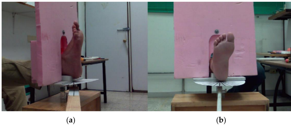
Figure 3. Foot posture during the image acquisition. (a) Lateral view of the foot on the resting base with angle and the thermal insulating foam background. (b) Frontal view. It is noteworthy that the pink background foam is large enough to isolate the foot from the remaining body of the volunteer so that the IR radiation does not interfere with the captured frame.
