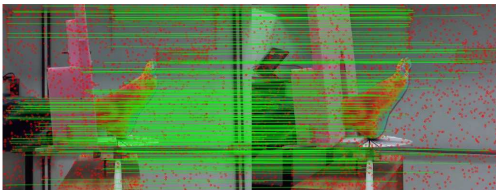
Figure 19. Detected feature points (red dots) and visualization of their correspondence (the green lines represent the link between homologous points). This figure represents 202 matches between images 6 and 7 from set S1, in which most of the key points were dismissed, proving that the quality of the model depends on the accuracy of the matching points' process.
