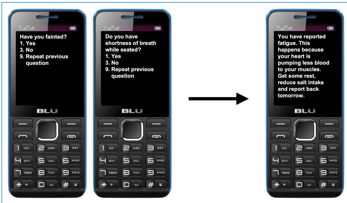
Figure 3. Simulated screenshots of the USSD workflow and resulting SMS message. SMS: short message service; USSD: Unstructured Supplementary Service Data.
