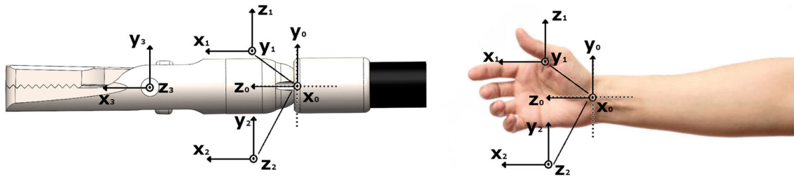
Fig. 2 The coordinate frames of the end effector that the handle is intended to manipulate, and the corresponding frames on the wrist
