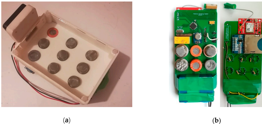
Figure 4. View of the assembled low-cost multi-sensor device in the stages of development: (a) prototype sensors, and (b) modified sensors.
