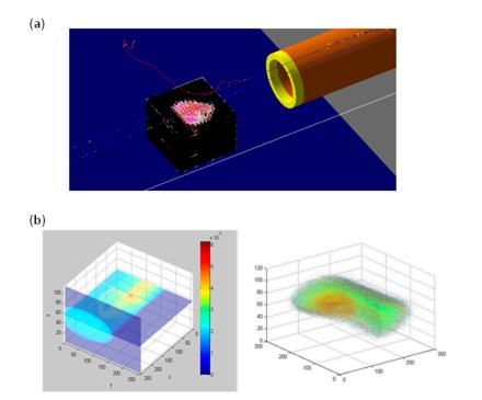
**Figure 1.** (a) Screenshot of DICOM volume in GEANT4. (b) Example of dose distribution calculated by Monte Carlo application.
