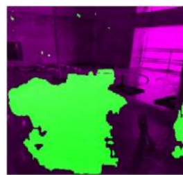
Figure 9. Examples of segmented images from the thresholding approaches (bright green: concrete; deep purple: non-concrete).
