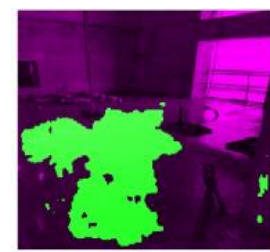
Figure 9. Examples of segmented images from the thresholding approaches (bright green: concrete; deep purple: non-concrete).
