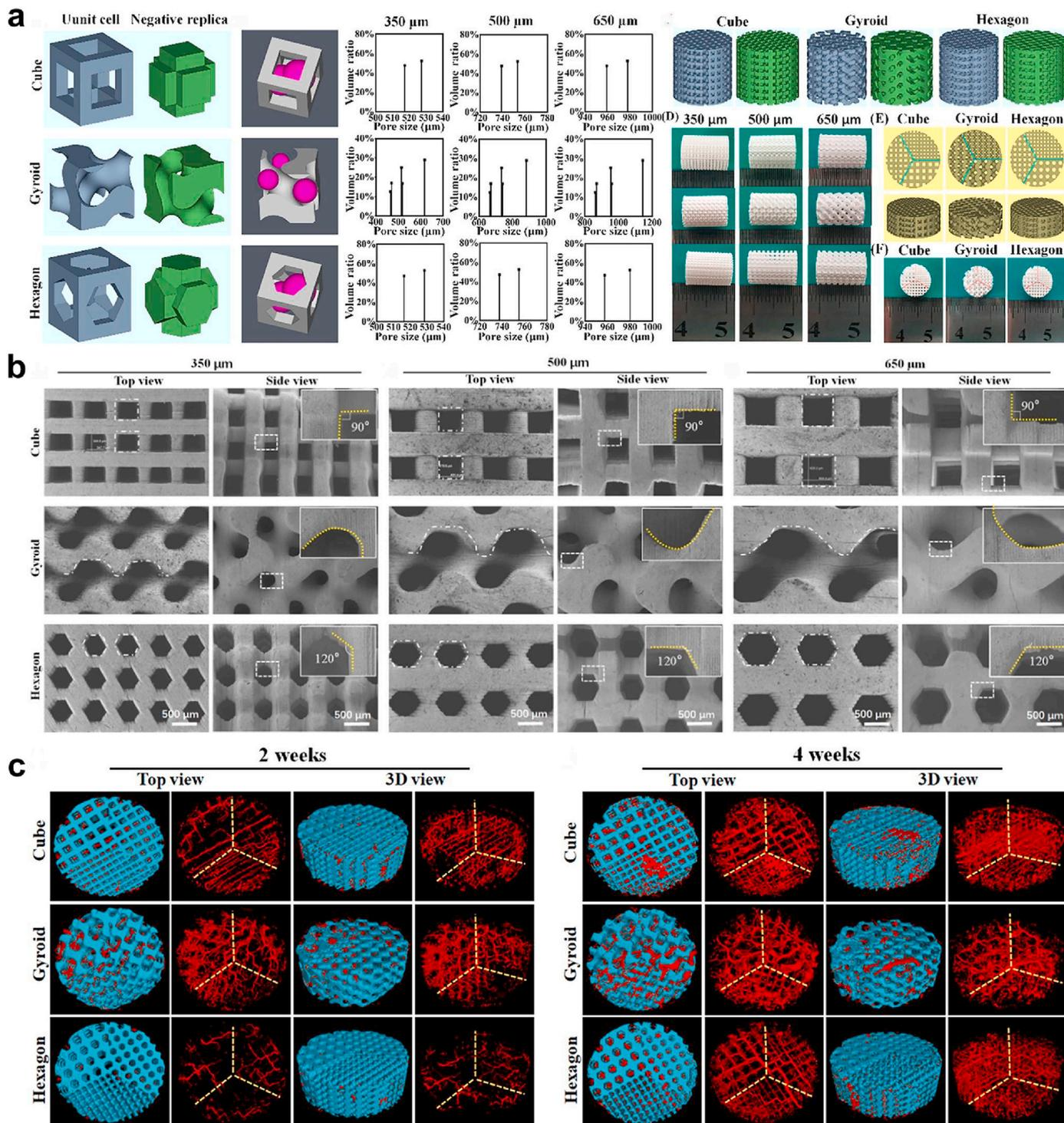
Fig. 6. a) Three-dimensional modeling and preliminary characterization of scaffolds with different hole geometries. b) Scanning electron microscopy (SEM) images of the surface morphology of bioceramic scaffolds with different pore geometries. c) Microangiographic images at 2 and 4 weeks after implantation [27].
