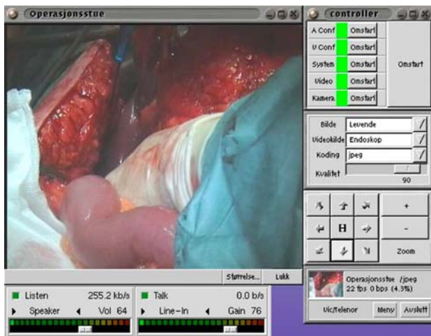
Fig. 6 Surgical telementoring. The remote control includes pan/zoom of a camera, giving overview images of the operating theater and pan/zoom of a camera mounted in the operation lamp. The system can switch between open and laparoscopic surgical procedures
