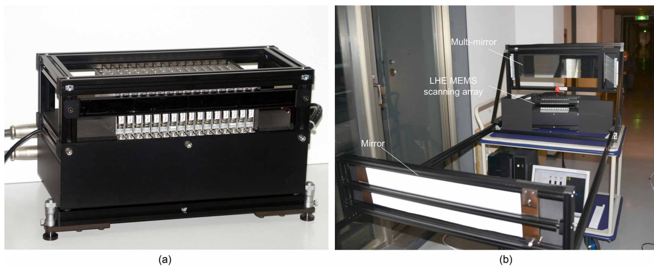
Figure 3 | Manufactured LHE 3D display. (a) Manufactured LHE 3D display with 16 MEMS scanning units; (b) LHE 3D display system using MEMS scanning array and mirror array for evaluation of long viewing distance 3D image.
