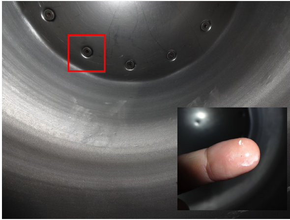
Figure 2. A finger swipe around the screw (red square) on a seemingly clean surface after cleaning and sanitation showed how easily operators could miss critical areas, which could become reservoirs that harbor microbial growth.
