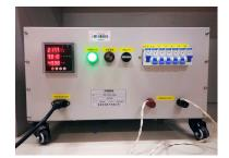
Figure 26. Adjustable resistance load box.
