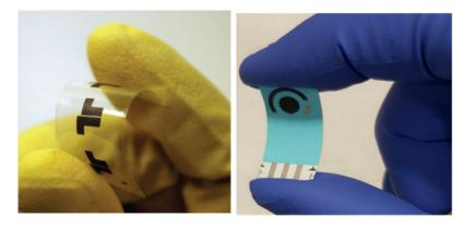
**Figure 12.** (Left) A real life image of micro-supercapacitors on a flexible polyethylene terephthalate (PET) substrate. Reproduced from [137] with permission from The Royal Society of Chemistry. (**Right**) A real life image of a pH sensor using melanin on a polyethylene (PE) substrate. Reproduced with permission from Tehrani et al. [121] under Creative Commons Attribution—Published by IOP Publishing.
