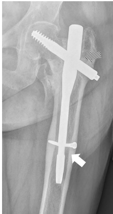
Fig. 5 A case of self-dynamism: breakage of the distal screw (white arrow) followed by a fracture of the nail (shadow arrow)
