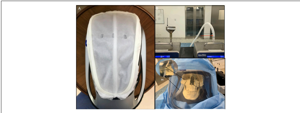
Figure 1. (A) Filter medium affixed on top of the Stryker helmet. (B): 2 TSI AeroTrak portable particle counters were used to collect the particles during the experiment; red broken arrow points toward the PVC tube that collected particles from inside the helmet; black solid arrow points toward the particle counter that collected particles from outside the helmet; (C): Stryker T5 helmet with the hood; inset (b) shows the flexible PVC tube affixed near the nose of the skull. Abbreviation: PVC, polyvinyl chloride; TSI, thermo-systems incorporated.
