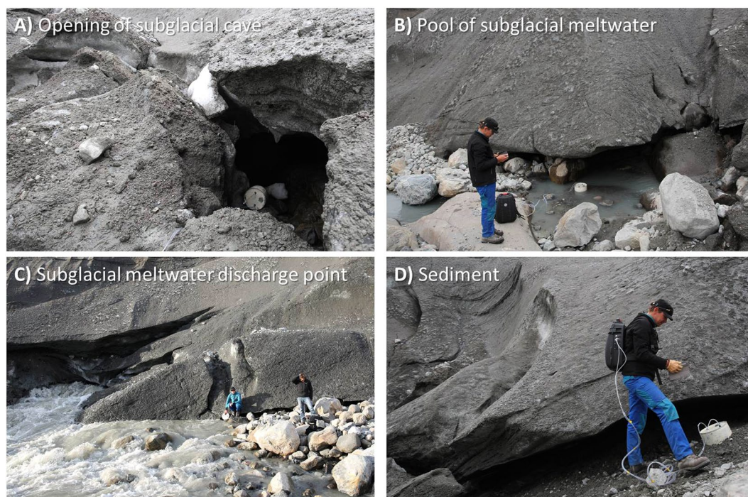
Figure 3. Modes of \text{CH}_4 and \text{CO}_2 measurements at the subglacial discharge point. (A) Open chamber inside the subglacial cave, (B) Closed chamber placed in a pool of subglacial meltwater, (C) open chamber placed in front of an ice crack connected to the subglacial discharge point and (D) Closed chamber placed on sediment beneath the ice edge. For (B,D) the chamber was connected to the analyzer forming a closed recirculation system for the measurement of the meltwater/sediment atmosphere exchange of gases, respectively. The mobile \text{CH}_4 and \text{CO}_2 analyzer (G4301, Picarro Inc.) can be seen in (B–D).
