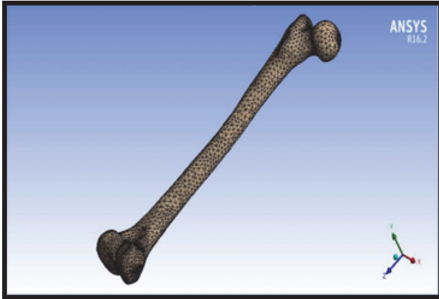
FIGURE 10: Meshing with tetrahedral elements.
