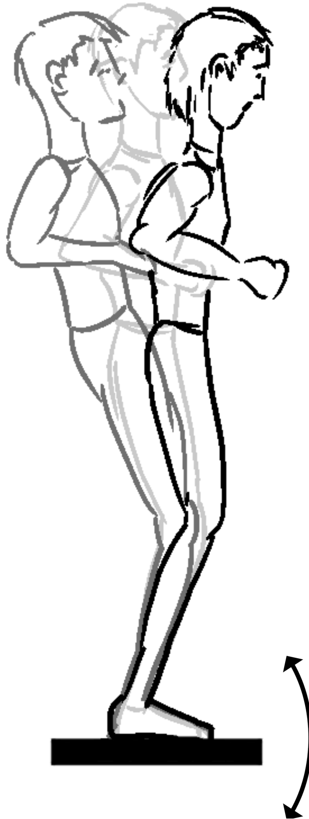
Fig 6. Rotating platform method with sudden or continuous pitch perturbation.
