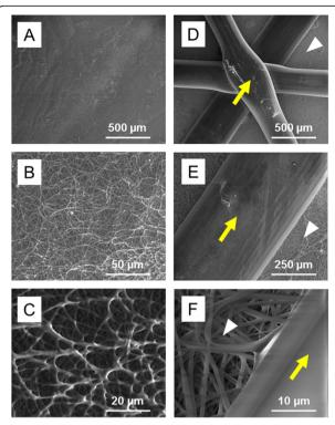
**Fig. 2** SEM imaging of reinforced electrospun scaffolds. **a-c** SEM images of the electrospun side of the reinforced scaffolds. Images show a uniform distribution of randomly oriented fibers. **d-f** SEM images of the 3D-printed side of the scaffolds. High magnification images (**f**) show that there is minimal damage to the electrospun fibers in the immediate vicinity of the 3D-printed PLA mesh. Yellow arrows depict the 3D-printed PLA. White arrowheads depict the PCL:gelatin scaffold
