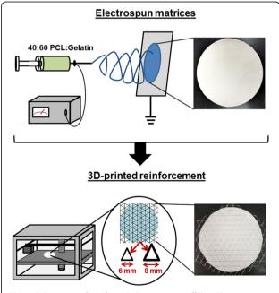
**Fig. 1** Fabrication of reinforced electrospun scaffolds. Electrospun scaffolds were produced from a 40:60 ratio of PCL:gelatin. The scaffolds were then placed in a 3D-printer and a PLA mesh was deposited onto one side of the scaffold. Two types of 3D-printed meshes were generated, one with a 6 mm distance between PLA struts, and the other with an 8 mm distance between struts
