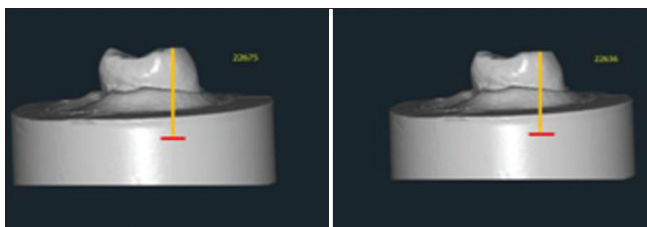
Figure 5: Auto computer-aided design scans showing teeth wear after 1 lakh and after 1.5 lakhs cycles
