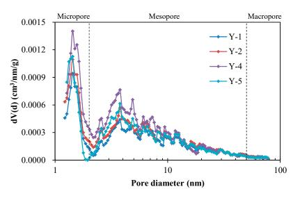
**Figure 6.** Pore size distributions (PSDs) obtained from N<sub>2</sub> adsorption isotherms of four shale samples (Samples Y-1, Y-2, Y-4, and Y-5).
