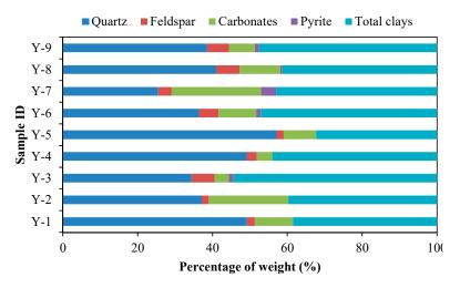
Figure 2. Mineralogical compositions of the shale samples.
