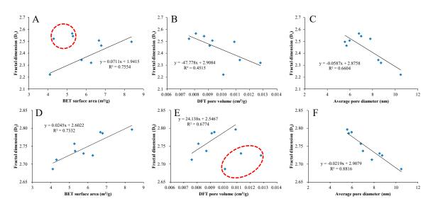
**Figure 13.** Plots of fractal dimensions D<sub>1</sub> and D<sub>2</sub> versus BET surface area (**A**,**D**), DFT pore volume (**B**,**E**), and average pore diameter (**C**,**F**).
