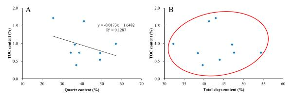
**Figure 3.** Plots showing the relationships of TOC content with quartz content (**A**) and total clays content (**B**) of the shale samples.
