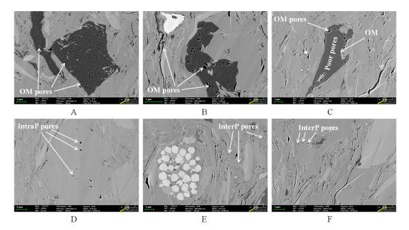
**Figure 4.** Field emission scanning electron microscopy (FE-SEM) images of micro-nanometer scale pores of the shale samples: (**A**,**B**) Abundant OM pores, (**C**) Heterogeneous OM pores characteristics in the same OM particle, (**D**) Abundant intraP pores, (**E**) Abundant interP pores between the clay minerals particles, (**F**) Abundant interP pores between the brittle minerals particles.
