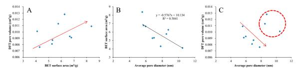
**Figure 8.** Relationships between density-functional-theory (DFT) pore volume and Brunauer–Emmett–Teller (BET) surface area (**A**), BET surface area and average pore diameter (**B**), DFT pore volume and average pore diameter (**C**).
