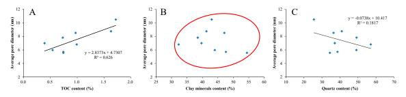
**Figure 11.** Plots of average pore diameter versus TOC content (**A**), clay minerals content (**B**) and quartz content (**C**).
