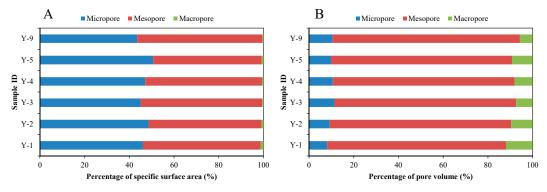
Figure 9. Percentages of specific surface area (A) and pore volume (B) of six typical shale samples.
