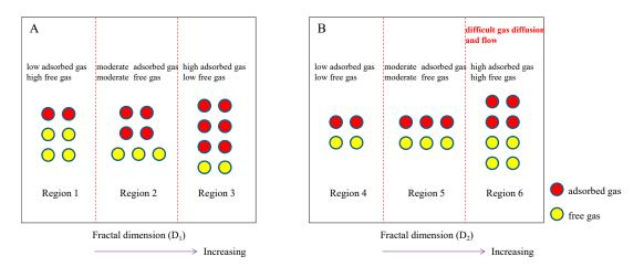
Figure 15. Relationships between shale gas storage capacity and fractal dimensions: (A) D<sub>1</sub>, (B) D<sub>2</sub>.
