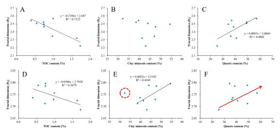
**Figure 12.** Plots of fractal dimensions  $D_1$  and  $D_2$  versus TOC content (**A**,**D**), clay minerals content (**B**,**E**), and quartz content (**C**,**F**).
