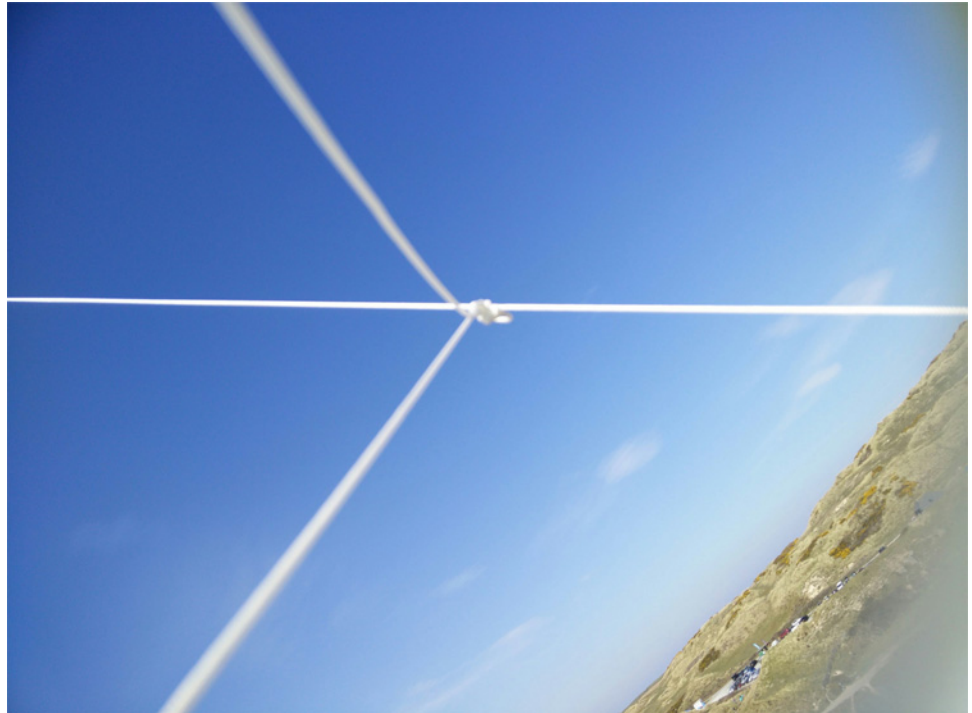
Fig 11. Example 'kite line' image captured with the OnePlus One phone from the KAP rig when the phone holder became inverted during a gust of wind.
