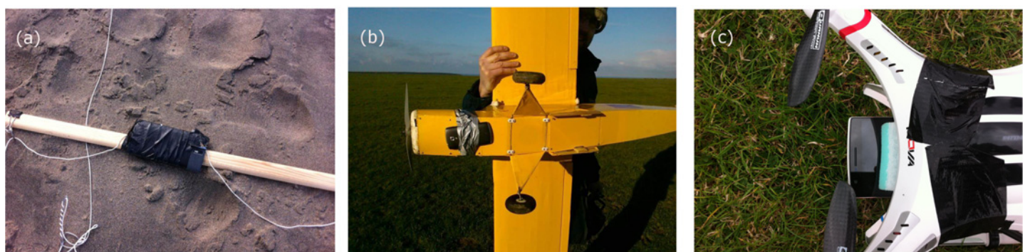
Fig 2. Examples of basic fitting methods to hold the mobile phone handset in place on airborne platforms. Shown are (a) a wooden bar suspended from two strings on the flexifoil stunt kite with the OnePlus One phone attached using hardware tape (b) the Acer Liquid Z3 taped to the underside of the balsawood Flair Cub aircraft with hardware tape and (c) the OnePlus One phone attached using hardware tape to the underside of the Quantum Nova lightweight quadcopter with a sponge to reduce image blurring caused by airframe vibration.
