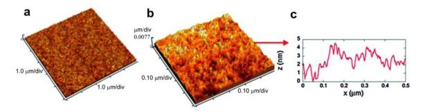
Nanotubes obtained on the granular surface of alumina substrates grew as a bunch of tubes on every grain. On the flexible substrate the same tube growth behavior did not take place due to the low roughness of the substrate, thus the surface roughness of the substrate also has an appreciable influence on the morphology of the resulting TiO<sub>2</sub> tubular arrays.
