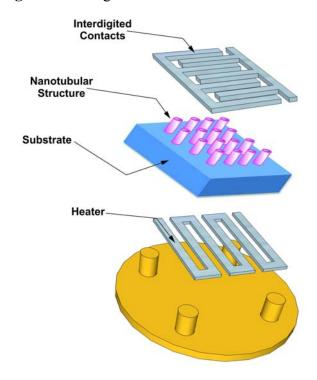
Figure 14. Design of a conductometric transducer.
