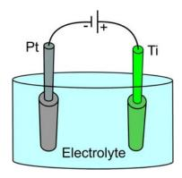
Preparation of titania tubular arrays by means of the anodization method in chromic acid solution both without and with hydrofluoric (HF) acid addition was performed for the first time by Zwilling *et al.* in
