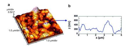
The surface analysis of the substrates showed a surface structure of stiff substrates composed by grains (alumina with the granular morphology) with measured sizes ranging from hundreds of nm to 1 µm (Figure 8), giving the substrate an RMS (root mean square) roughness of about 105 nm. Differently, the flexible polymeric substrate showed an almost flat surface (Figure 9) with an RMS
