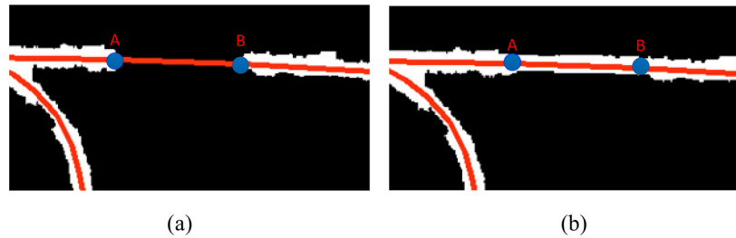
Fig 6. (a) two disconnected road segments (red line segment is OSM road); (b) linking result.
