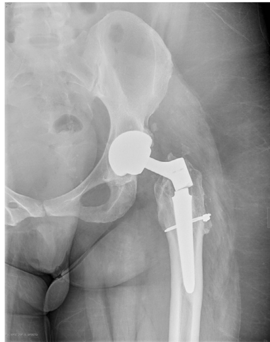
Figure 3. Neck-stem junction breaking in 1st revision implant after atraumatic pain two years after the revision. The rupture is localized on the thread at the neck-stem junction. The neck was virus (135°) in Ti6Al4V.
