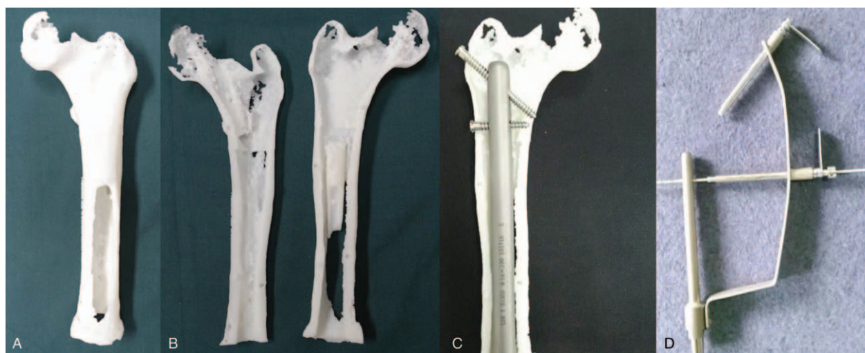
Figure 5. Three-dimensional (3D) printed model matched with customized prosthesis and navigator. A, The residual femur. B, The residual femur in halves. C, Assembling test. D, Navigator design.
