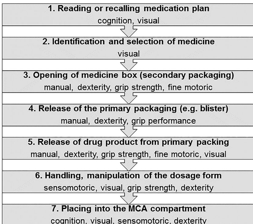
FIGURE 2 Task decomposition and chronological sequence of the medication preparation process and the major human capabilities required. MCA, multicompartiment compliance aid
