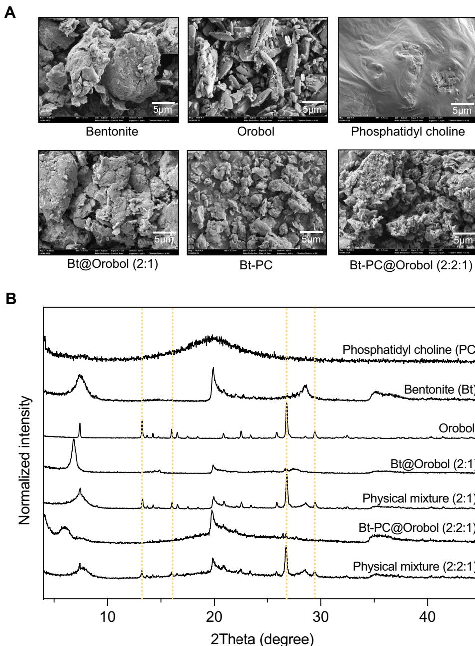
**Figure 4** Physicochemical characterization of orobol-loaded bentonite composite formulations. **(A)** FE-SEM images of bentonite, orobol, phosphatidylcholine and bentonite composite formulations. The scale bar is 5  $\mu$ m. **(B)** pXRD of PC, bentonite, orobol, bentonite composite formulations and physical mixtures.
