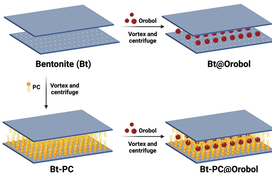
**Figure 1** Schematic illustrations of the preparation process of Bt@Oroborol and Bt-PC@Oroborol composite formulations. Oroborol and PC were loaded in the Bt@Oroborol and Bt-PC@Oroborol formulations based on the adsorption mechanism.<sup>7,10,19</sup>
