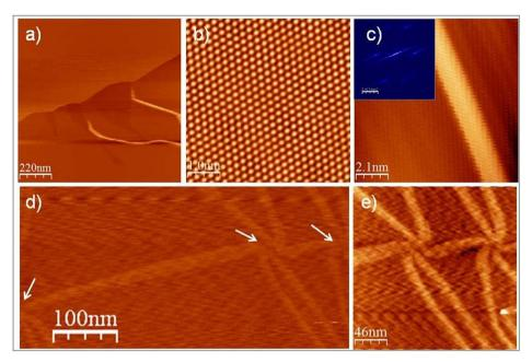
Figure 2 | Morphology of trilayer graphene. (a) Large STM image (-1.7 V, 1 nA) of trilayer graphene (b) Triangular type structures  $(5 \times 5 \text{ nm}^2)$ , (c) An STM image of corrugated graphene with nearly periodic ripples of nanometer wavelength (inset Fourier transform of the STM image) (d) STM image of three interconnected flower-shaped structures, (e) STM image of two interconnected flower-shaped domains.  $V_s = 0.05 \text{ V}$ ,  $I_t = 200 \text{ pA}$ ) for (b - e).
