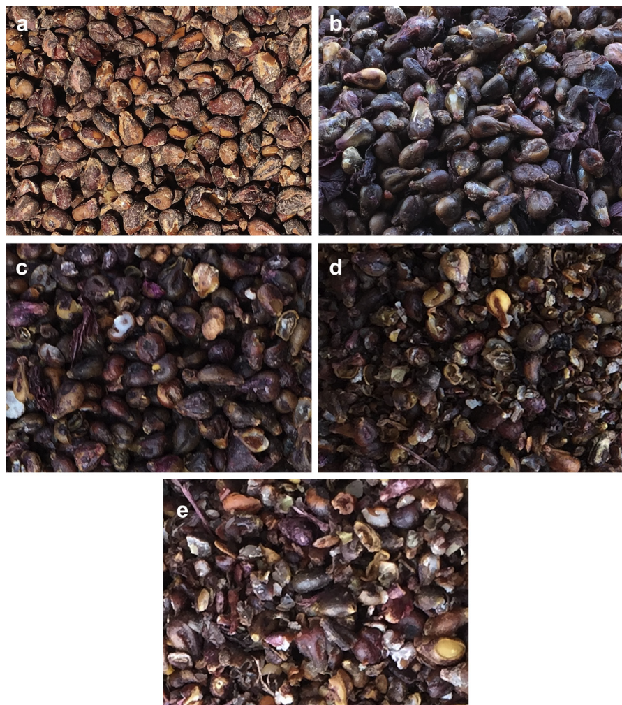
Fig. 7. Comparison of seeds of the control (a) and the seeds obtained by Type- B blade settings at: b) 480 rpm; c) 576 rpm; d) 672 rpm; e) 864 rpm.
