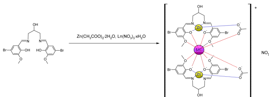
Scheme 1. Scheme of synthesis of trinuclear coordination compounds Zn^{II}-Ln^{III}-Zn^{II} ( Ln = Nd (1), Sm (2), Eu (3), Tb (4), Dy (5)) of N,N' -bis(5-bromo-3-methoxysalicylidene)-1,3-diamino-2-propanol ( H_3L ).
